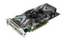
The FX 5500 graphics board is an ultra high-performance professional graphics solution for CAD, DCC, and visualization applications. Engineered to address the most demanding GPU challenges, the NVIDIA Quadro® FX 5500 by PNY features: 33.6GB/sec. memory bandwidth and a 256-bit memory interface with support for 1024MB ultra-fast GDDR2 memory, two dual-link DVI connectors, and resolutions up to 3840 x 2400.
